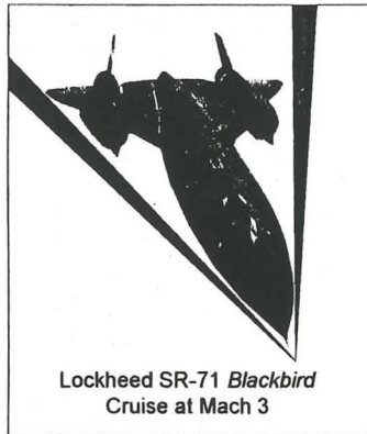
The highly swept rear mounted wings of the SR-71 Blackbird
